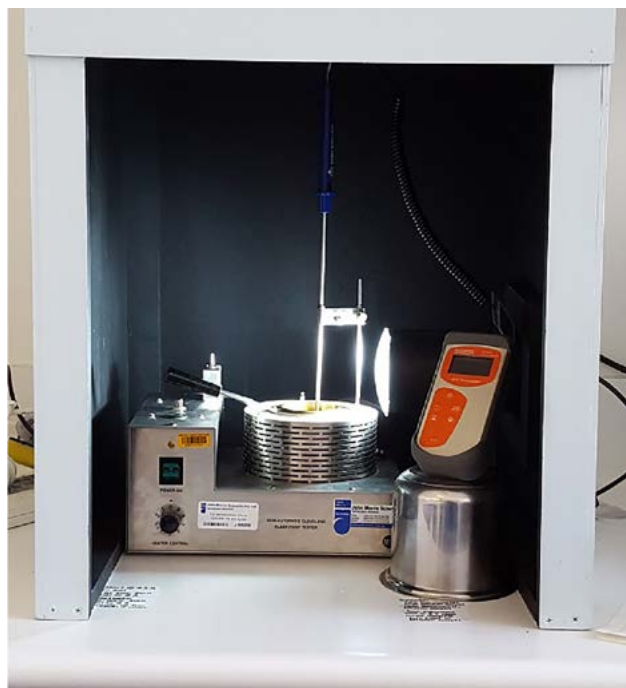
A wooden box with appropriate ventilation and a built-in light source helped to prevent air draught, to help with the Determination of a derived smoke point for olive oil (OL15000)
