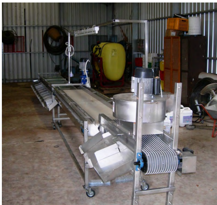
Figure 9: A mechanised table olive sorter and grader
