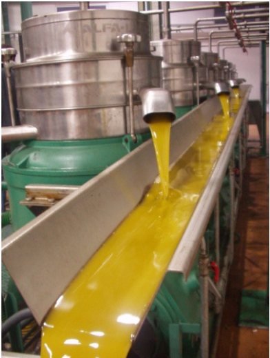
Vertical separators clarifying the oil
