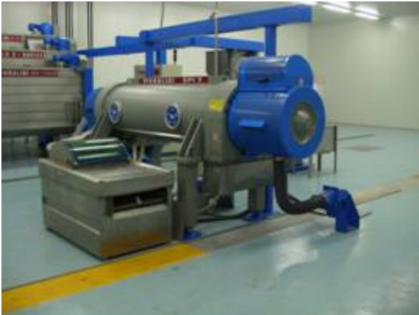
Decanter separating olive oil from paste
